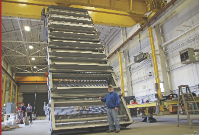
Multirake Bar Screen for Port Monmouth at our Orange Facility
